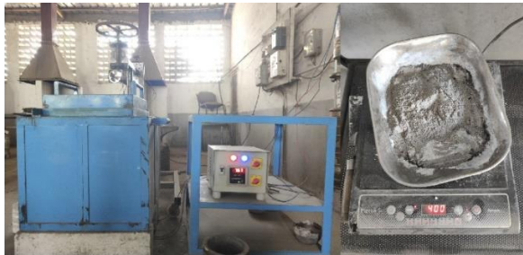
Fig4.3: Stir casting and reinforcement preheat set-up
